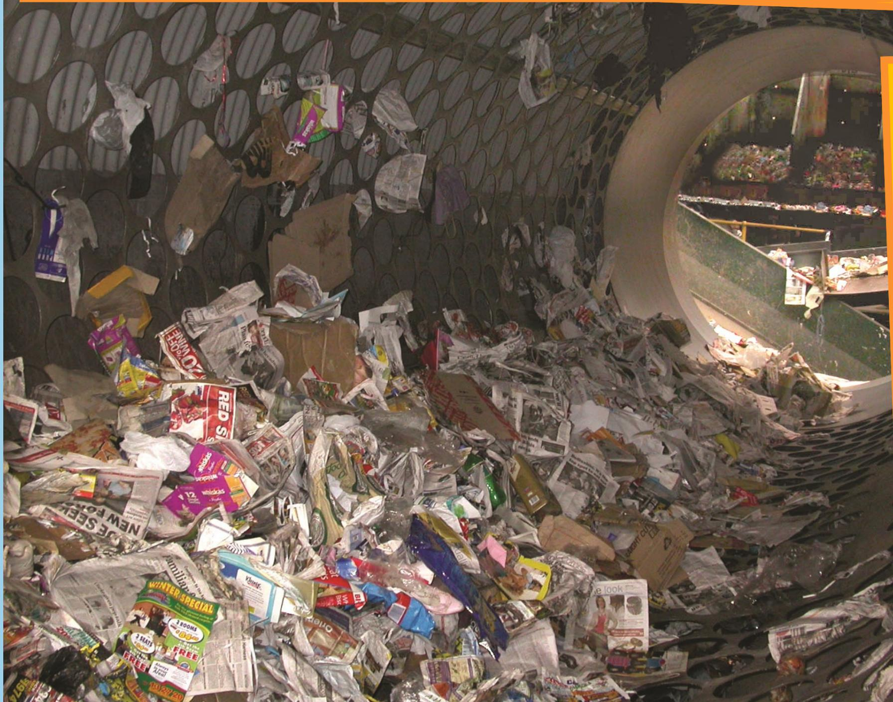
The trommel has holes and as it turns, containers, bottles, cans and jars fall through the holes. Flat things like paper come out the other end.
